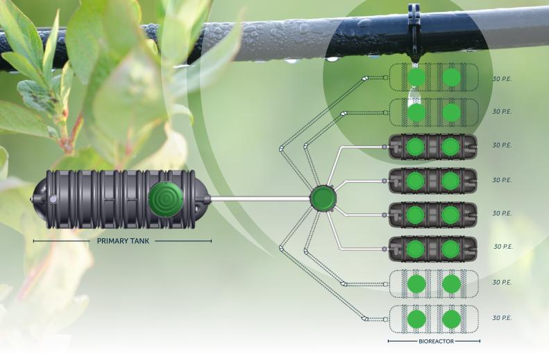
When the ECOROCK units are installed in parallel they can accommodate up to 240 P.E.
